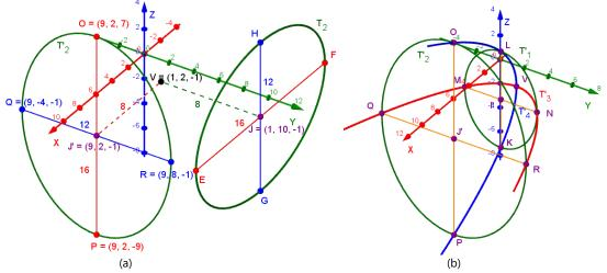
Figure 12. Representation of paraboloid S2 through dimensional deconstruction of S1
